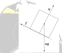
6. Remember, components of forces MUST NOT be drawn on the free body diagram of any body !!!
